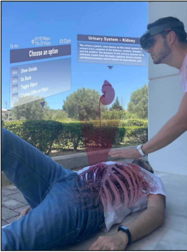
Fig. 1. The PPDR responder uses an AR HMD to see overlaid info and deformable objects on top of the patient. Envisioned example of UI layout.
