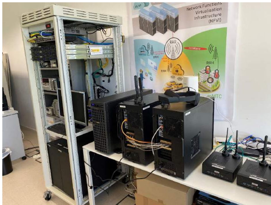
Figure 13: Part of the CTTC 5G testbed showing some of the servers and the Amarisoft 5G equipment
